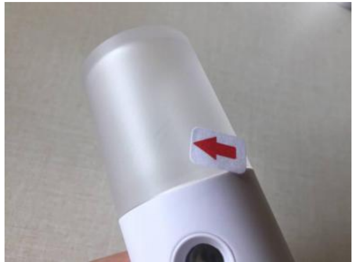
Scratch mark on plastic bottle
