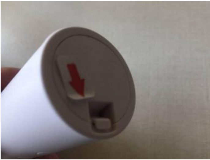
The battery cover assembly no smooth
